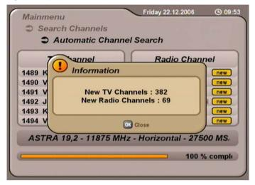
Press the OK button. You will be asked whether you wish to save the changes or not. Selection is performed using the AV buttons and is confirmed using the OK button. If you select "Yes, save changes", the newly found channels will be added to the end of the channel list. Then press the EXIT button to exit the menu. The channel list is called up on to the TV screen by pressing the OK button (see also section "On-screen displays" "Channel list TV/Radio").
